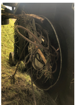
Mower blade entangled with cable left in ditch.
