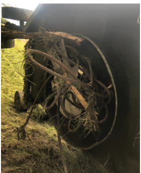
Image: Smoky Lake County mower received damage after it was tangled up in a cable that was dumped in the road right of way.
