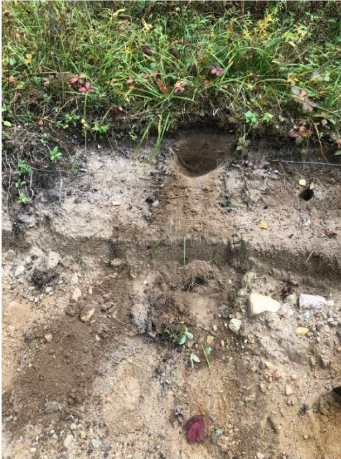
Photo 3. Greater view of soil profile at TH6, shallow litter/topsoil overlying sandy subsoil material and followed by the target sand and gravel deposit.
