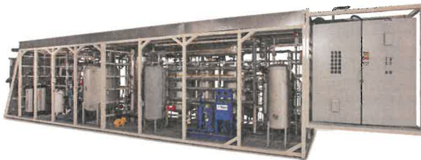
Figure 28 – Syn Gas to Diesel Fuel Processing Module
