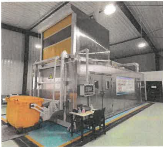
Figure 16: Bin-fed Version of Shredding Module
